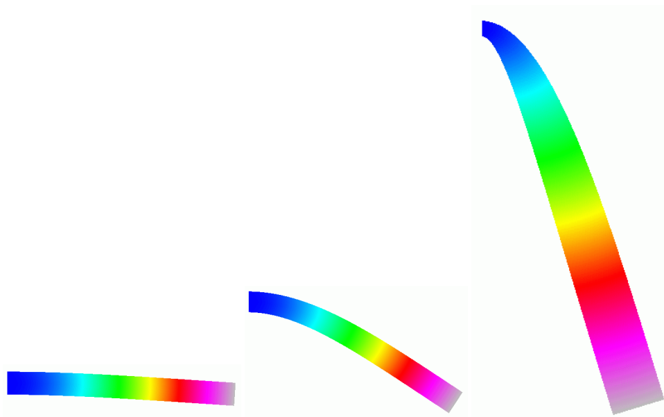
Figure 29.2: The displacement of an elastic beam with different loads using a linear model
